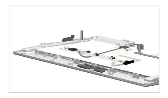
Figure 5-41. Disconnecting the EasyPoint II Controller
